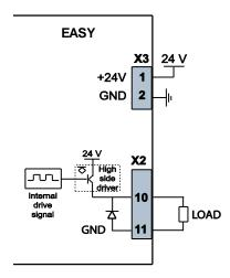
Digital outputs can be paralleled in order to increase the maximum output current. Be careful to connect all paralleled outputs to the same drive signal.
