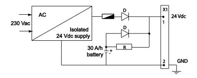
The EASY drive consumption is less than  $300 \, \text{mA}$  with  $24 \, \text{V}_{DC}$ . So, a  $24 \, \text{V}$  /  $30 \, \text{A/h}$  battery can keep the drive powered during e.g. a long 3-day week-end. This backup method is interesting for saving the machine initialization as well as the axis position even when moving with the mains switched off.
