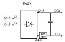
Note: The soft start system remains operational when the drive is powered by the DC- and DC+ inputs.
