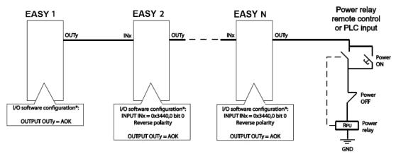
Note: Maximum delay for the power relay deactivation: number of EASY drives x 1ms.
