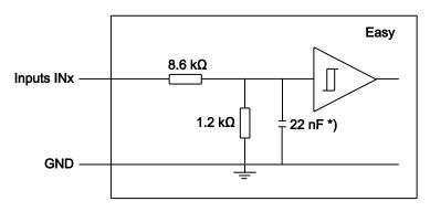
$^{\star}$ ) From serial number 11420004, the capacitor value is 10 $\mu$ F for the IN4 input only, in order to support safety relays with test pulse output (for short-circuit detection).
