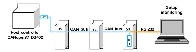
RT = 1200hm terminal resistor connected between CAN-L and CAN-H lines
