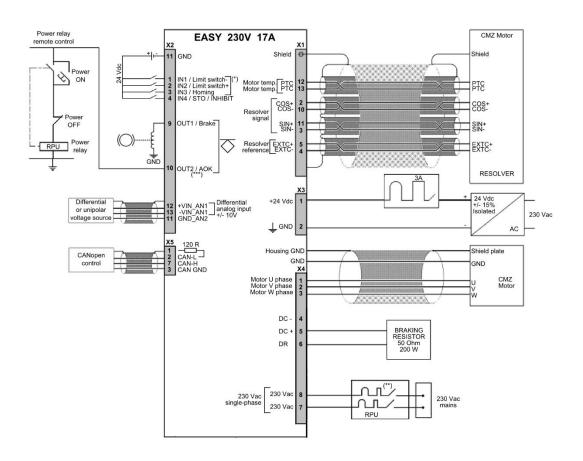
**Note:** The 24V and power supplyprotection on source side must be ensured by the user.
