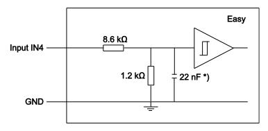
\*) From serial number 11420004, the capacitor value is 10 μF for the IN4 input only, in order to support safety relays with test pulse output (for short-circuit detection).
