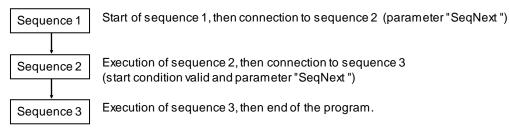
If the execution is starting at sequence 1 and logic input 8 is deactivated, the program will be the following:
