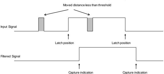
Capture of motor position while motor running with a logic input signal
