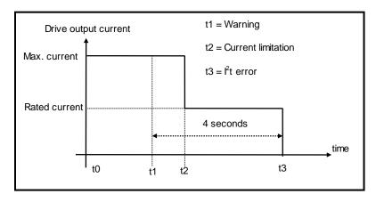
The maximum current duration before release of the warning is depending on the value of the parameters **Rated current** and **Max. current**. This value is calculated as follows:
