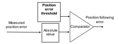
The measured position error value is continuously compared with the **Position error threshold** parameter value. When the measured position error is exceeding the **Position error threshold**, the position following error is released. This configuration is used for applications requiring the smallest possible following error.
