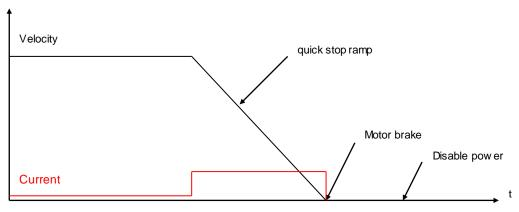
Stop 3 - stop on current limit: the motor is slowed down in velocity loop with a current limitation.
