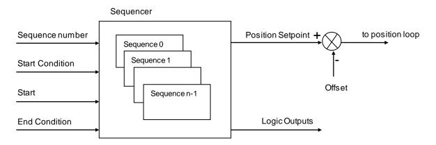
**Sequence Number**: allows the selection of the sequence to be executed. The "Sequence Number" can be connected to physical logic inputs or set via the fieldbus to select the sequence.
