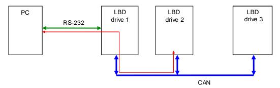
The **LBD** drive supports Node ID setting by GemDriveStudio software: menu "Tools", sub menu "Node ID setting". Node ID value must be unique for each drive connected on the fieldbus. Node ID range is from 1 to 63.
