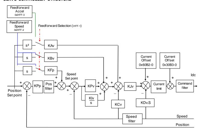
**Speed loop** gains are the most critical to adjust because they greatly depend on the mechanical load characteristics (inertias, frictions, coupling stiffness, resonances,...).
