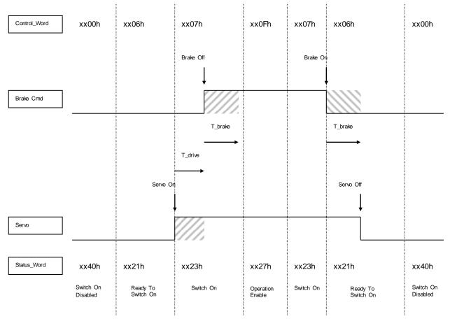
T\_brake: Motor Brake Reaction Time
