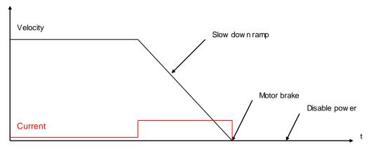
Stop 2 - stop on speed ramp: the motor is slowed down in speed loop with a quick stop speed ramp. The initial speed is defined with the current motor speed.
