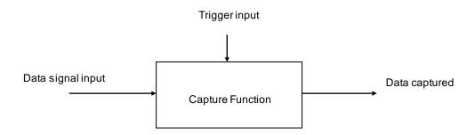
The purpose of the capture function is to latch a data signal (generally position value from a sensor) on a trigger input signal (generally a logic input).
