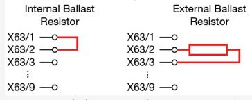
How to connect a braking resistor to the X40 PSD1-M\_P supply:
